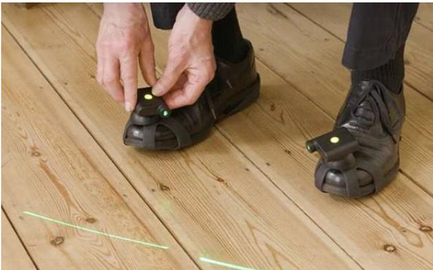
The Path Finder exploits this by using a small laser that clips on to the shoe and projects a green line in front of the foot, replicating the idea of having a stair to climb.
